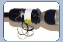
Actuate drill to remove jacket and expose the center conductor, then make sure the final cut is in the valley.
