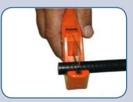
Straighten cable. Use RDCUT-TER-S, applying even pressure around cable while rotating tool around cable to cut off cable squarely.
