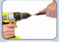
Use the coring bit "U" to remove dielectric until cable reaches stop on tool. You may optionally use the included T-Handle to prep/strip and core cable.
