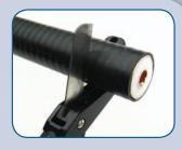
Straighten cable and position RDCUTTER in valley of corrugation and cut off cable squarely.
