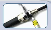
Stabilize connector with adjustable wrench and always be sure to torque the mating connector.
