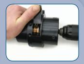
Make sure blade is positioned over valley closest to end of cable, release blade lever and actuate drill until cable is completely cut.
