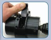
Attach prep/strip tool to drill. Open blade lever and lock with pin. Insert cable and actuate drill.
