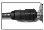
Slide the WPS-5 over the JMA 7/8" DM connector, making sure to overlap the dedicated 7/8" port seal. WPS-5 should overlap to cover grooves.
