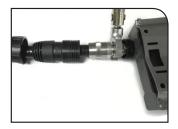
Torque the connector to 18 ft. lbs. using the TQ-114-F18 torque
