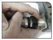
Pull the dedicated 7/8" port seal over coupling nut. Seal should cover nut.
