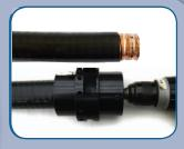
After stripping again, cable is ready for connector measurement marking. **Three** full visible ridges are acceptable. See that the cut is made in the "valley."
