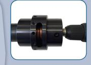
Re-apply stripping tool to remove one more corrugation of jacket for three full visible ridges.
