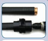
Blade lever is shown fully closed. Open lever, lock with pin, and remove tool. Two ridges should be visible.
