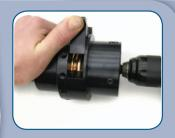
Make sure blade is positioned over valley closest to end of cable, release blade lever and continue until cable is completely cut.
