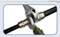
When using the torque wrench, make sure the mating connector is supported by an adjustable wrench.
