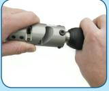
Attach prep/strip tool to drill. Keep the prepped cable end at a downward angle during the prep/coring process.
