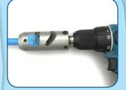
Actuate drill to remove jacket and expose the center conductor, then make sure the final cut is in the valley.
