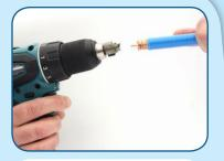
Use the coring bit "PL" to remove dielectric until cable reaches stop on tool. You may optionally use the included T-Handle to prep/strip and core cable.
