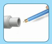
Hold prepped cable end at a downward angle, tapping the cable while vacuuming a second time.
