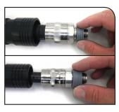
Prep the 1/2" cable and install the 1/2" connector. Refer to the UXP-12 installation instructions. Install the port seal provided onto the N female connector. This seal is gray in color & marked "for use with connector".
