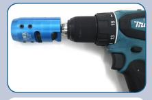
Attach prep/strip tool to drill. Be sure you are using an SP-12S tool.
