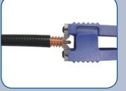
Use center conductor cleaner ("SP-CC tool") to remove any remaining dielectric material on center conductor.
